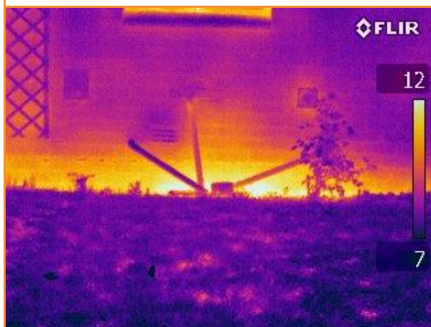
6.35: Thermographic images showing leakage along base of kitchen wall
