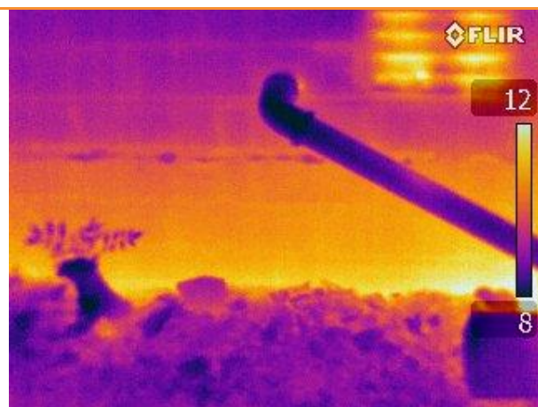
6.35: Thermographic images showing leakage along base of kitchen wall
